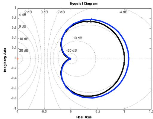
Figure 10: The Nyquist plot of the augmented plant – does not cross the negative real axis.
