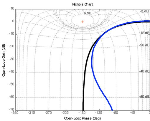
Figure 12: The Nichols plot of the augmented plant – does not deviate beyond  $-180$ deg at low frequency and  $-90$ deg at high frequencies.
