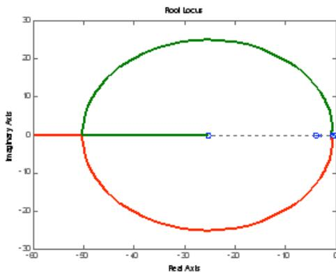
Figure 13: The Root Locus of the augmented plant – has only one asymptote.
