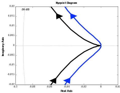
Figure 11: The Nyquist plot of the augmented plant zoomed near the origin – reaches the origin from  $\pm 90$ deg directions.
