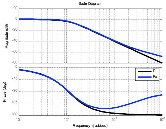
Figure 9: The Bode plot of the original plant,  $P(s)$ , and the augmented plant,  $P_a(s)$ .
